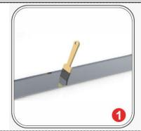
Clean the sundries on the installation surface, ensure that the surface is clean.
