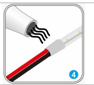
Use the heat fan to blow the heat shrinkable tube at the welding position until the heat shrinkable tube shrinks and wraps the welding position
